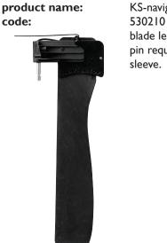
KS-navigator rudder, pin 42 mm blade length 500 mm pin requires separately sold rudder
